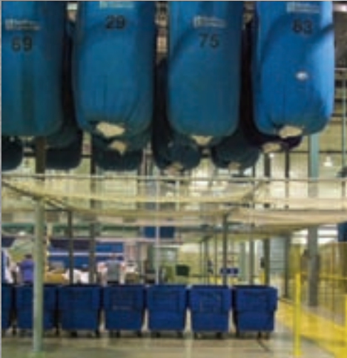
Soiled linen is stored in large bags on an automated future rail system and sorted by type. The bags are then transferred to a specified station for processing. This design reduces the need for manual movement of linen in carts on the plant floor and reduces congestion.
